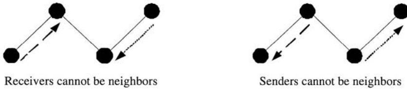
Figure 3: 802.11: Spatial reuse with CSMA/CA
